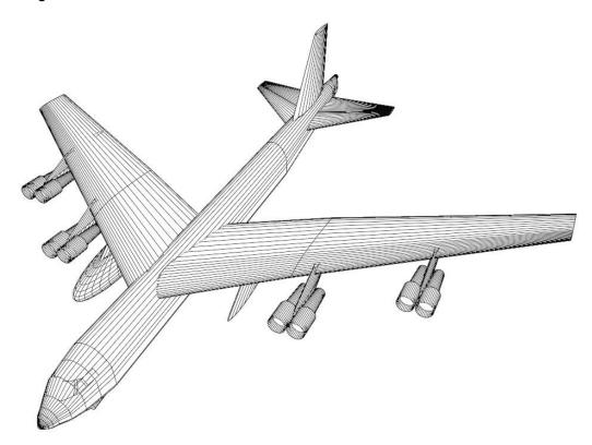
First flown in 1952, the B-52 forms the backbone of the USAF strategic bomber fleet. Most significant improvement of the final B-52H variant are the Pratt & Whitney TF33 turbofan engines instead of turbojets of the earlier models. Heavy load capacity and long range make the B-52 a good base for special variants such as mothership for air-launched vehicles.
