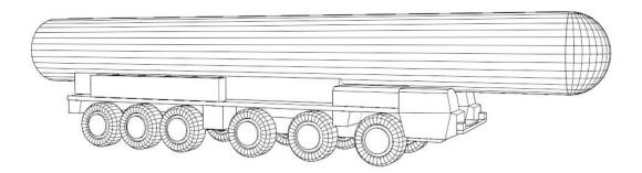
Transporter-loader vehicle for 5Ya27 long range missiles of the S-225 ABM system. Based on the MAZ-547 12x12 heavy truck chassis. Positions missile launch canisters vertically on static launch mounts.
